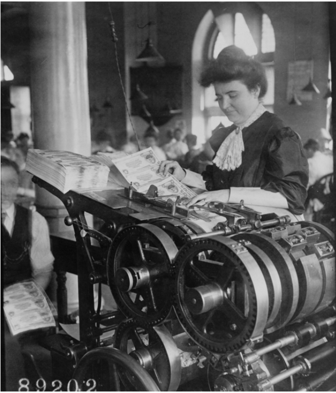
Figure 2a. An operator feeds uncut sheets of $5 third charter national bank notes into a high speed rotary numbering press.
