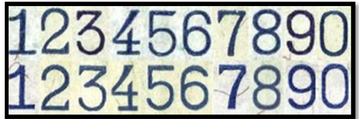
Figure 3. Comparison of the old style fonts from the single action machine (upper line) and the new style fonts from the high speed rotary press (lower line). Old style fonts are more closed in design. Note the distinctive droopy 2, hunchback 3 and long-handled 4.
