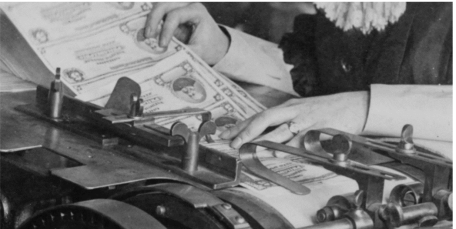
Figure 2b. Close up showing sheets being fed in top-down around a cylinder to receive the serial numbers from an opposing, outer cylinder.
